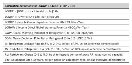
For multiple types of equipment, a weighted average of all base building HVAC&R equipment must be calculated using the following formula:
